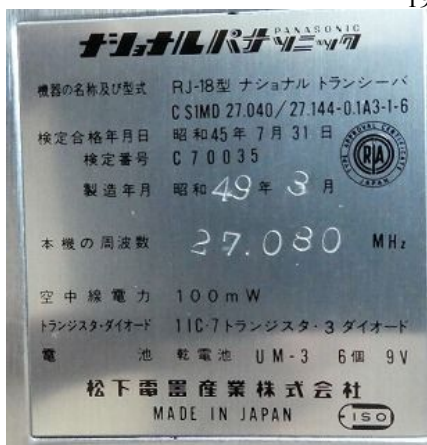
Fig. 3. RJ-18 Name plate. Manufactured in 1974. Power:100 mW, Freq. 27.080 MHz
