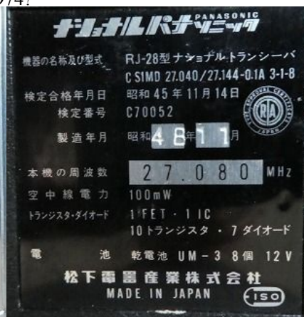
Fig. 4. RJ-28 Name plate. Manufactured in 1973. Power:100 mW, Freq. 27.080 MHz
