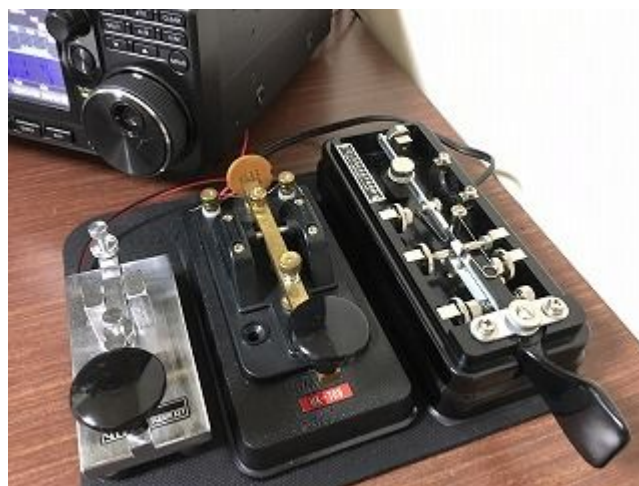
My keys, GHD GT-705A at the left, HI-MOUND HK-709 at the center, and BK-100 at the right, ICOM IC-7300 is for the CW mostly.
