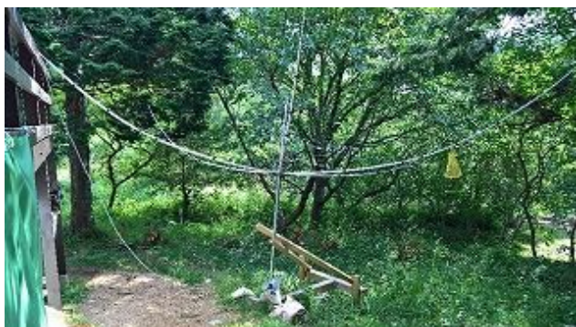
“Temporary” installation of HEX Beam on the Ground. Yellow marker so that I could confirm the HEX Direction via IP Camera on 2nd Floor Balcony when working my IZU Remote.
