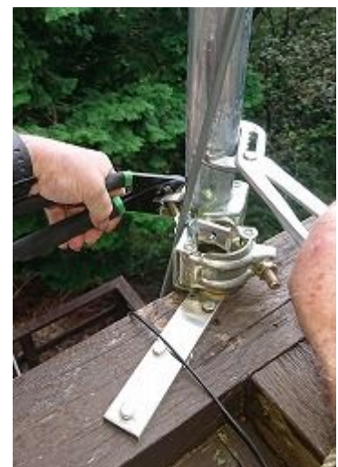
The scaffolding coupling serves as a brake and the grippers as my "ARMSTRONG ROTATOR". (Being close to my Operating Position - I can quickly rotate the HEX from the 2nd Floor Balcony)
