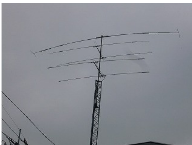
With the first grade, I operate DIGITAL (JT65/JT9/Other), CW and Phone now. My Rig TS-590G. My Antennas. Top:40m-30m DP middle:20m-15m-10m 2ele HB9CV bottom:17m-12m 2ele HB9CV and for 80m.
